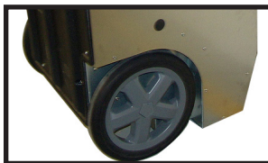
Inboard wheels allow for tighter storage and improve maneuverability.
