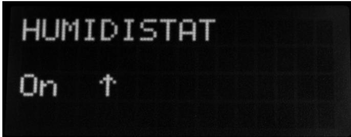
Press the Set button to toggle the Humidistat Mode On/Off. Press the Next button to advance to the next screen. If Humidistat mode is enabled, then proceed to Humidistat Set point. Else, proceed to Humidity Units.
