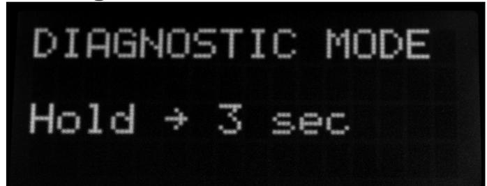
Press the Next button for 3 seconds to enter Diagnostic Mode. This action can also be performed at any time while the machine is powered on.
