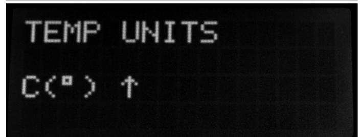
Press the Set button to toggle the temperature units between F (o) and C (o)
