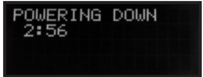
The default shut-down time is three minutes plus 20 seconds for a final purge. The shutdown time can be changed by scrolling through the menu to this screen.
