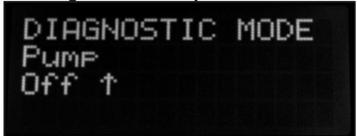
Press the Set button to toggle the Pump On/Off.
