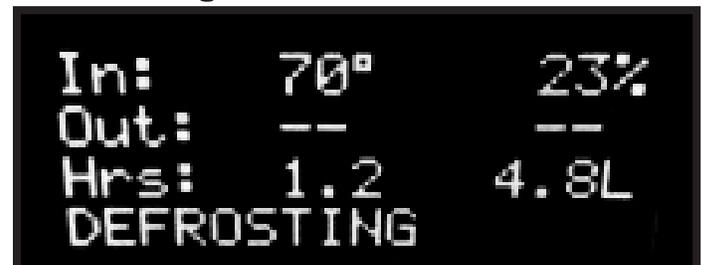
The display will communicate to the user that the machine is defrosting on the fourth line of the dashboard. This will momentarily replace grain depression until the machine has finished defrosting.
