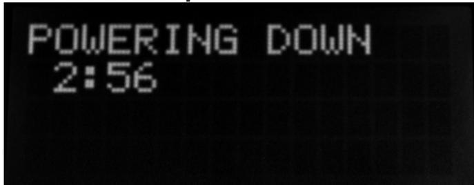
Press the Set button to adjust the shutdown time in one minute increments ranging from 3 - 20 minutes.
