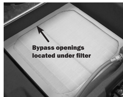
Remove filter, snap bypass cover into position shown, and replace filter.
