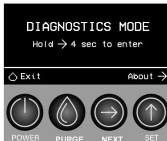
Press the Next button for 3 seconds to enter Diagnostic Mode. This action can also be performed at any time while the machine is powered on.
