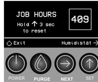
Press and hold the key for three seconds to reset the job hours from any screen.
