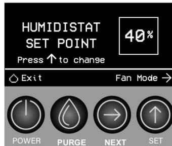
Press the Set button to adjust the set point RH% in 5% increments ranging from 20% RH to 80% RH and then looping back to 20% RH.
