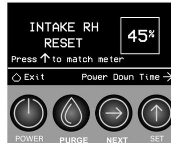
The Intake RH Reset allows you to calibrate the DryMAX to match your favorite meter. Use the Set Key to increase the reading on the screen with your meter.
