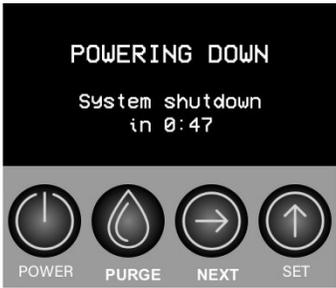
Press the Set button to adjust the Power Down Time in one minute increments ranging from 3 – 20 minutes.
