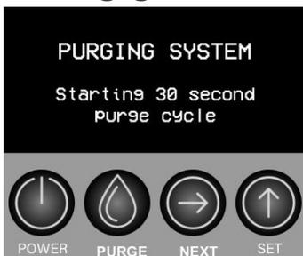
Press the PURGE button to purge the machine. The display will communicate to the user that the machine is purging on the fourth line of the dashboard and show a 20 second countdown timer. This will momentarily replace grain depression until the machine has finished purging.
