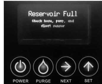
For help with the “Reservoir full: check float, pump, and hose” error see section 5.3 Troubleshooting
