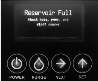
If the float is up for 60 seconds the status bar will turn red and the screen will display “Reservoir full: check float, pump, and hose”. To clear this error the float must go down.
