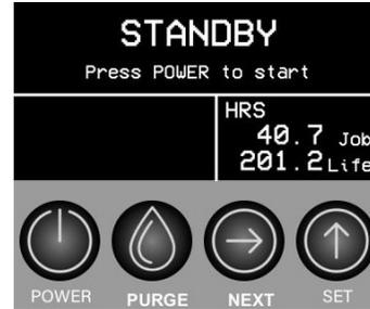
Press the button to turn the dehumidifier on. The unit will begin the Powering Up sequence and you will see this screen:
