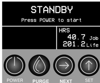
When plugged in but without pushing the power button, the display will communicate to the user that the machine is in Standby mode and ready to be powered on. In Standby Mode, the display will also show the current job and life hours on the fourth line.
