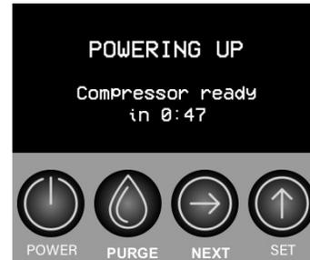
Press and hold the Power button to turn the dehumidifier off. The dehumidifier will go through a powering-down cycle.
