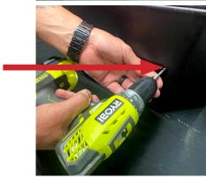
Using a T20 Torx screwdriver, remove the 4 screws securing the outlet grill in place.
