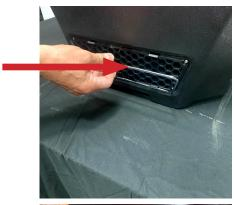
Remove lay-flat duct ring.
