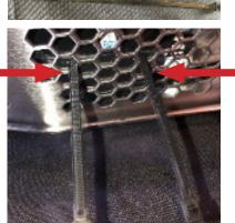
While holding the DryTAG RH sensor on its side against the inside of the exhaust grill, pass two zip ties through the openings of the exhaust grill and through the slots in the DryTAG RH sensor.
