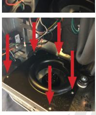
With the capacitor out of the way, remove the five screws attaching the inlet ring using a T25 Torx screwdriver.
