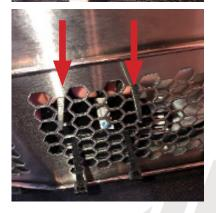
With the zip ties through the grill and sensor, lay the DryTAG RH sensor flat against the exhaust grill and pass the two zip ties back through the exhaust grill.
