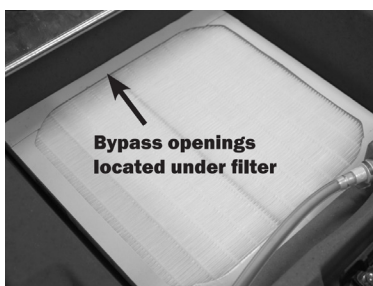
Figure 6: Remove filter, snap Bypass cover into position shown, and replace filter.
